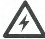
Caution: Risk of Electric Shock
