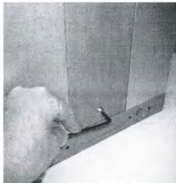
2. Remove single retaining screw.
