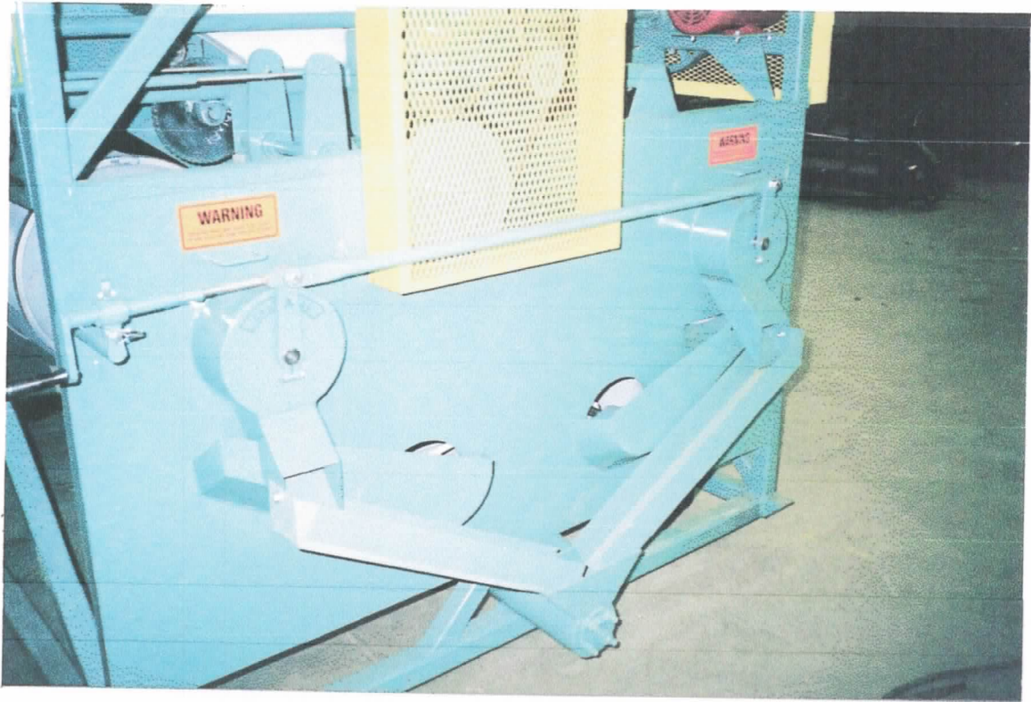
Screenings discharge and collection system.
