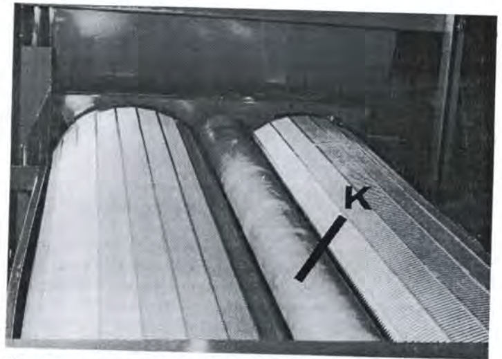
For proper operation, roll (K) must be in place to knock seeds out of the screen.
