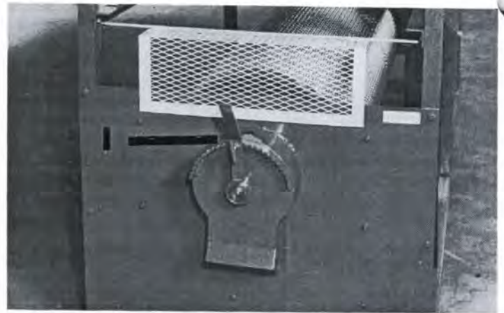
The trough in final portion of the indent can also be adjusted. Move lever (I) to select the notch to give the best seed selection.
