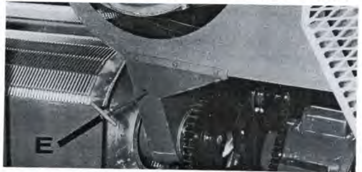
To evenly divide flow of grain into each cylinder, control rod (E) can be moved in or out.
