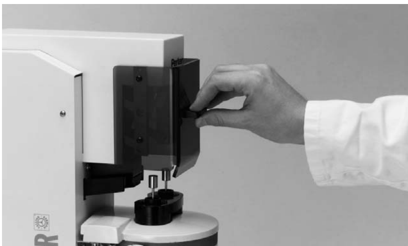
Figure 15. Pull down the plastic cover.
