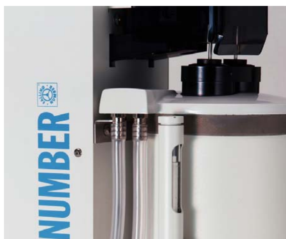
Figure 7. Connect plastic tubing securely to the cooling lid nozzles.
