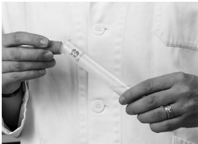
Figure 11. Scraping residues into tube rim.
