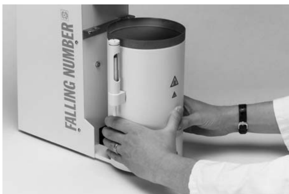
Figure 5. Fit the contact and slide in the water bath so that it is properly secured.
