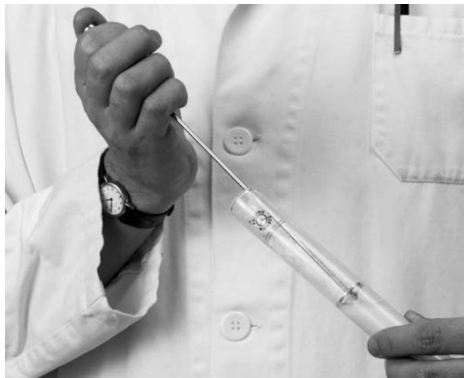
Figure 12. Scraping residues into suspension.
