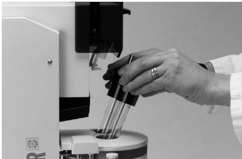
Figure 14. Place the cassette with tubes into the water bath.
