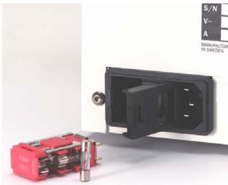
Figure X:1. Fuse holder removed and fuse coverlid open. (230V; 5x20 mm fuse)
