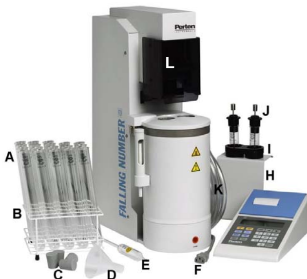
Figure 1. Falling Number apparatus model 1900 with accessories. L=Plastic cover
