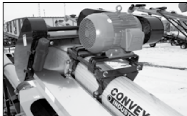
Fig 59 - Electric motor, speed reduction drive
