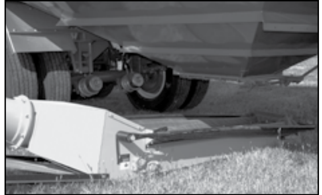
Fig 18 - Conveyor under truck
