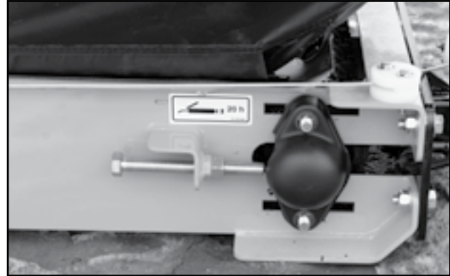
Fig 39 - Hopper roller bearing
