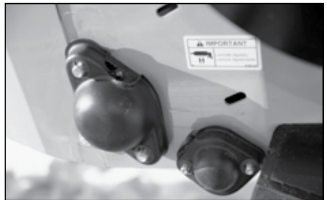
Fig 38 - Discharge roller bearings
