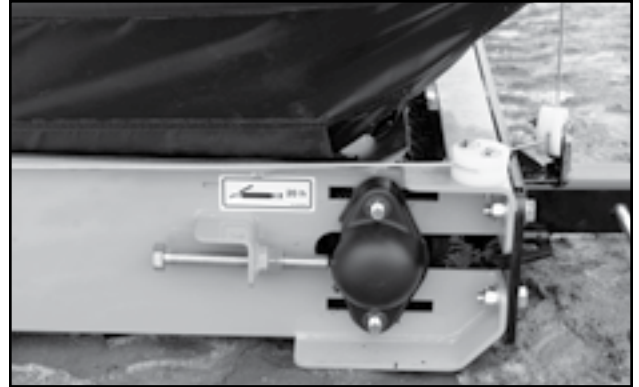
Fig 52 - Tail roller bearing housing
