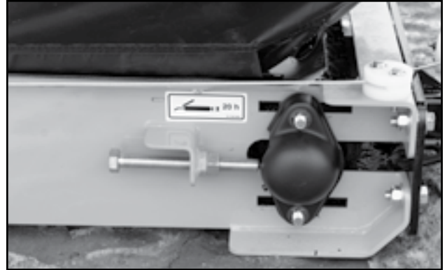
Fig 50 - Roller bearing mounts and anchor bolts
