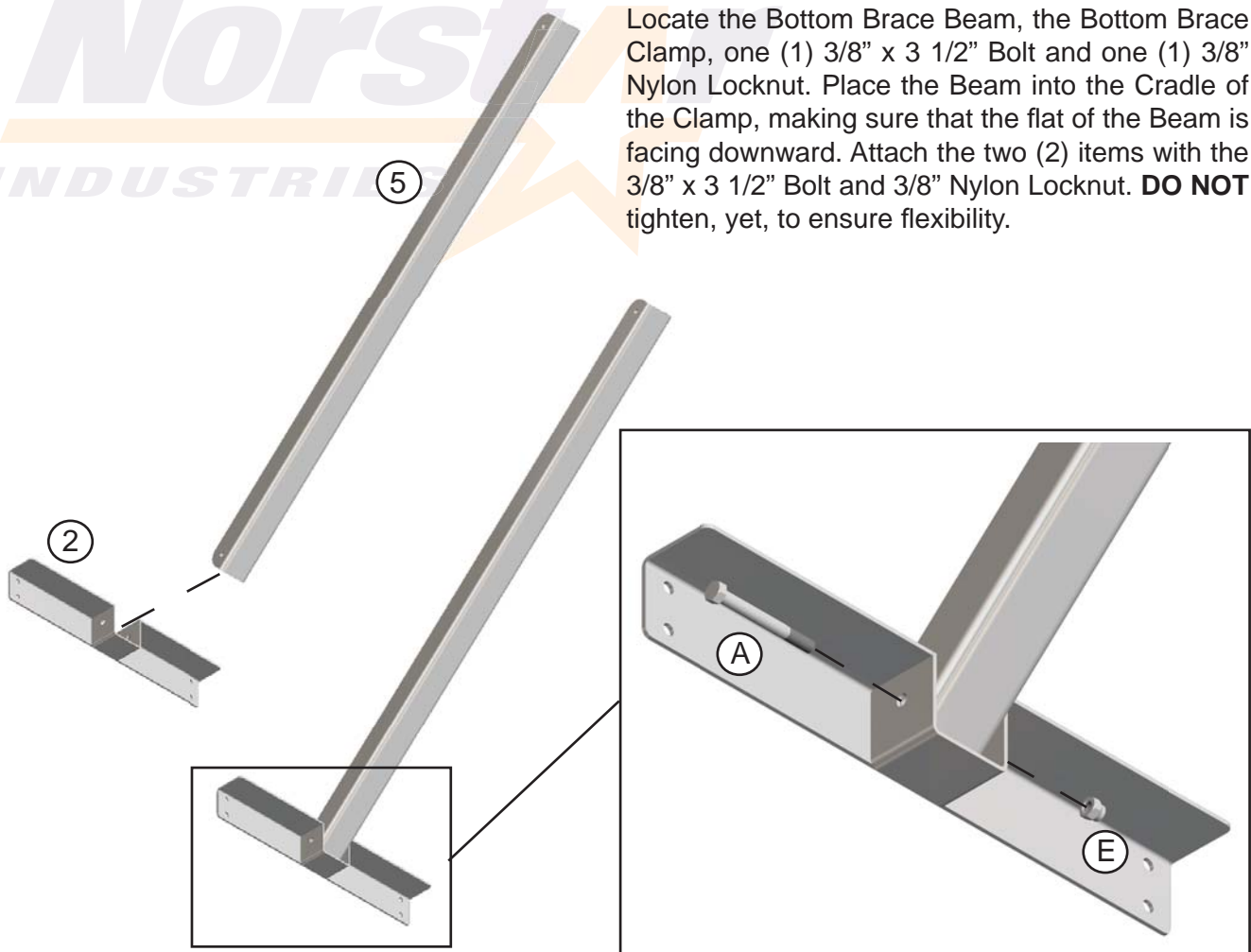
Figure 46 Bottom Brace Assembly
