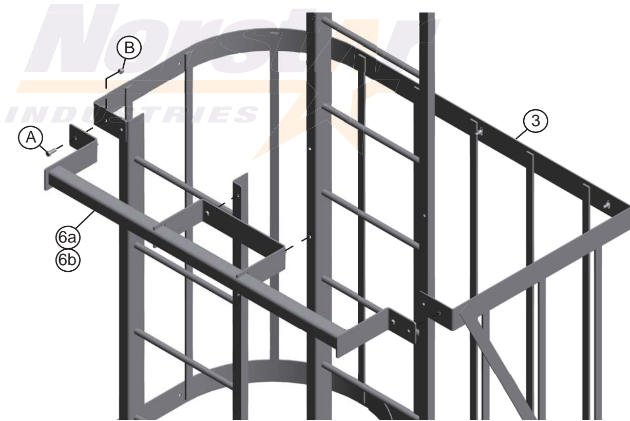
Figure 61 Trunking Clamp Bar Installation
