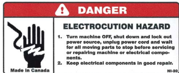
Figure 5 Electrocution Hazard Decal NI-20
